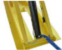
Safety device operating during lowering with acoustic signal activation
